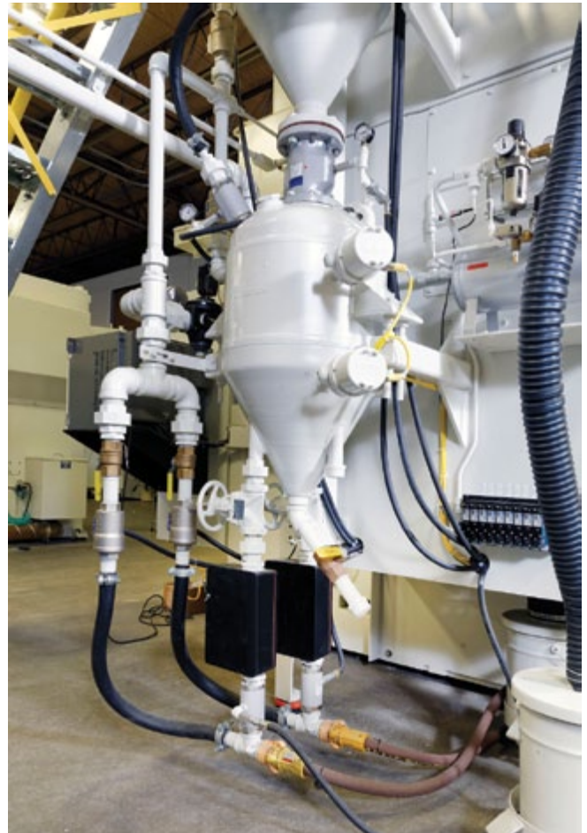
Each of the three Progressive Surface shot peening machines has two 700-24 MagnaValves for non-ferrous media.
