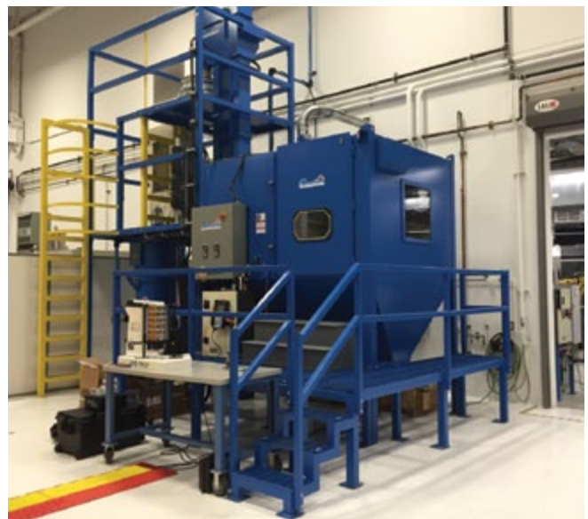
The shot peening machine at École Polytechnique de Montréal is used for academic research and testing projects for the aerospace industry in Montreal.
