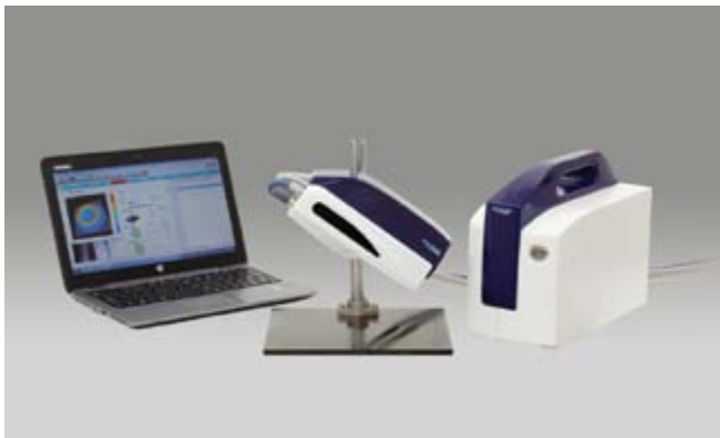
Figure 1. Residual stress measurement device ( \cos\alpha method).
