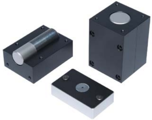
Figure 3. Standard specimen for residual stress measurement.
