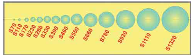
Fig.3. Size range of cast steel shot.
