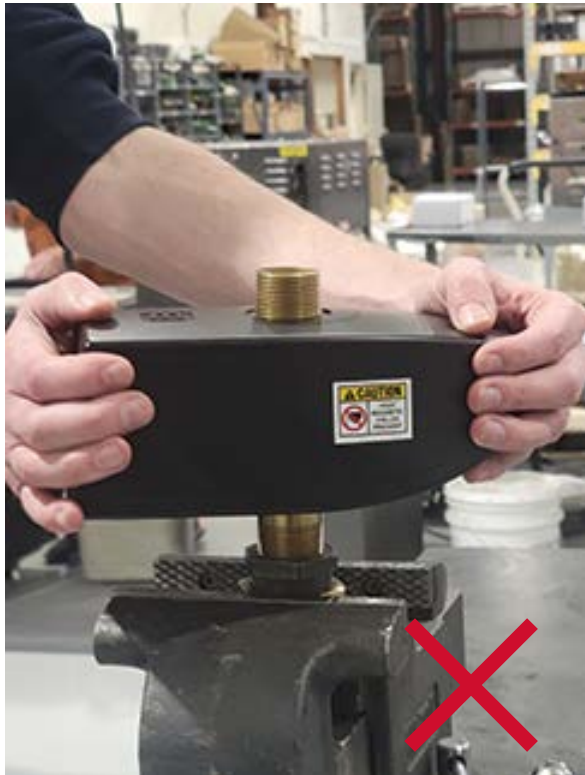
Do not use the valve body as a wrenching surface. This can break the valve.
