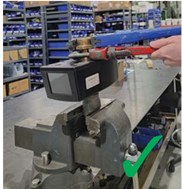
Do use two pipe wrenches—one on the valve pipe and one on the pipe fitting.
