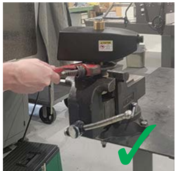
Do mount the pipe fitting in a vise and use one pipe wrench on the valve pipe to attach or remove the pipe fitting.
