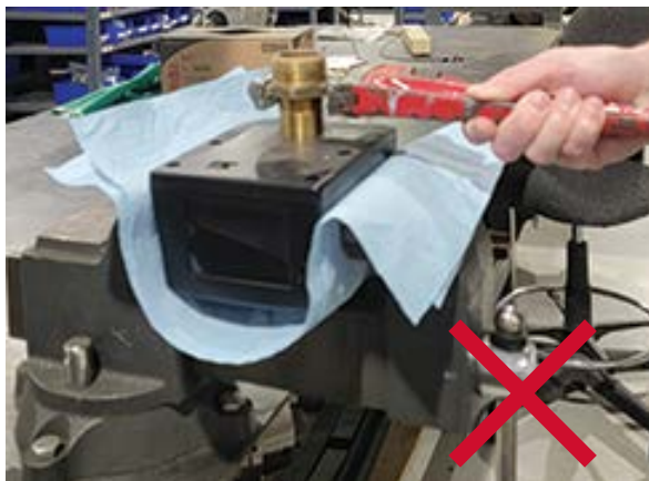
Do not mount the valve in a vise. Do not use a single pipe wrench on the pipe fitting.
