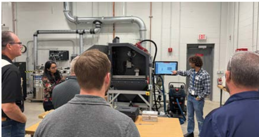
Langdon Feltner, a Purdue Graduate Research Assistant, reviews the capabilities of the senstenco shot peening test stand at a demonstration in Purdue's Manufacturing and Materials Research Laboratories.
