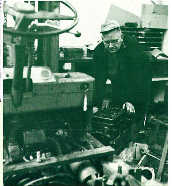
"Roundy" Feters replaces overhauled fork lift motor in new vehicle maintenance garage. The garage served as a coal bin before we converted to gas heat.
